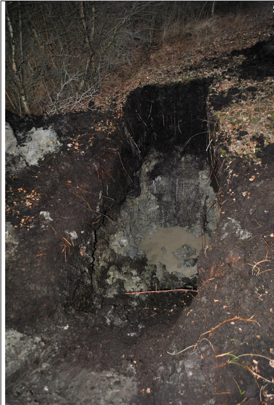
View of TP. Water trickling from the interface of peat and clay (continuous weak flow). Walls slightly unstable and crumbling (mostly on water path).
